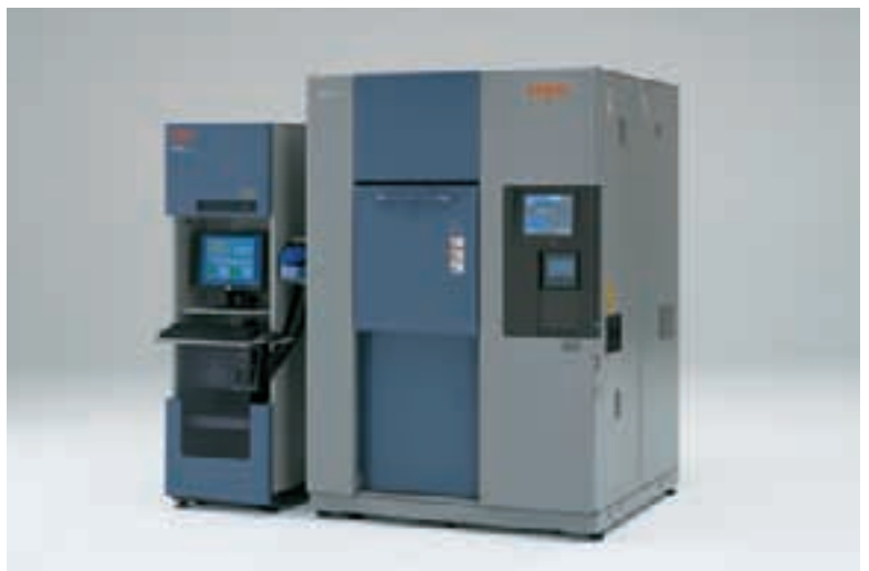
Example of the thermal shock chamber connected with the conductor resistance evaluation system
