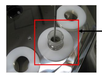
Set a nozzle in place so that its tip is placed in a position between the center and the edge of a flask.
